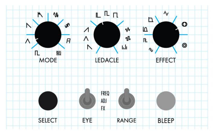
The T3k uses three knobs and a SELECT button to allow you to easily select and adjust many different parameters.
