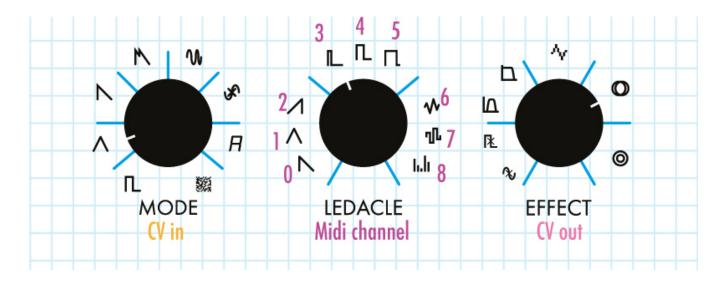
To change the MIDI input channel, have plug in the input jack. Same for output, even if you're using USB MIDI.
