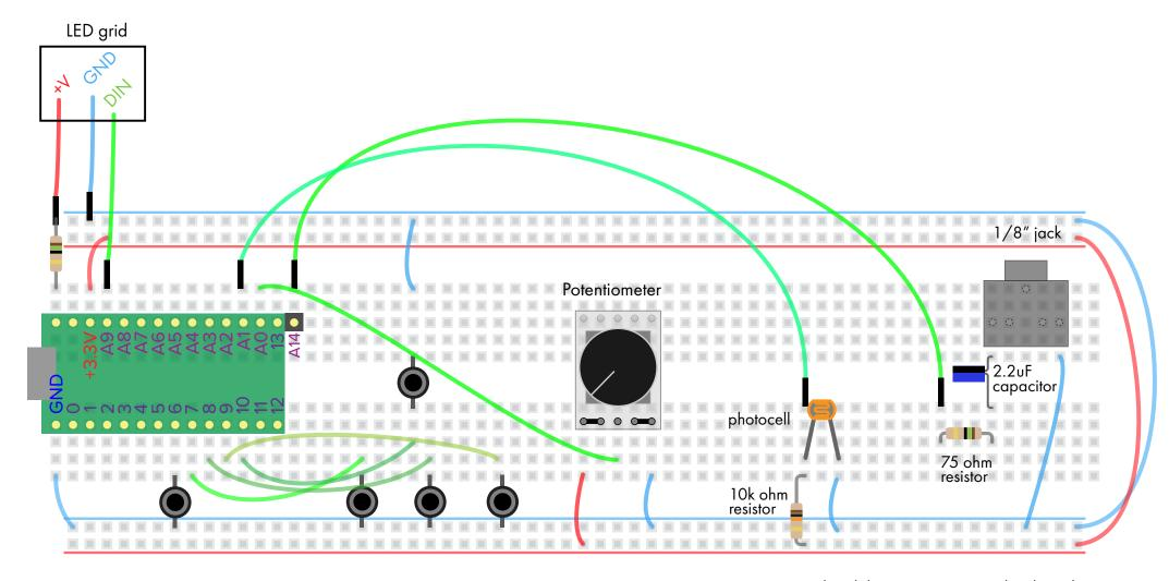
For headphones connect grond to the right most pin. For a mixer or amp connect ground to the middle pin
