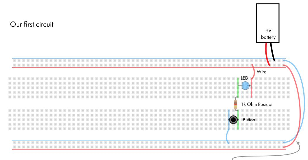
These wires connect the two "busses" on either side of the board
