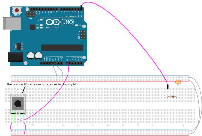
The first and second pins of the pot are connected together.
